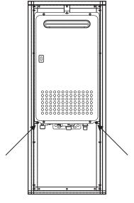
Figure 4: Location of lower mounting brackets.
