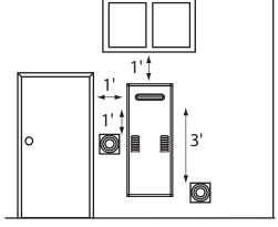
Figure 1: Discharge Vent Clearances.
